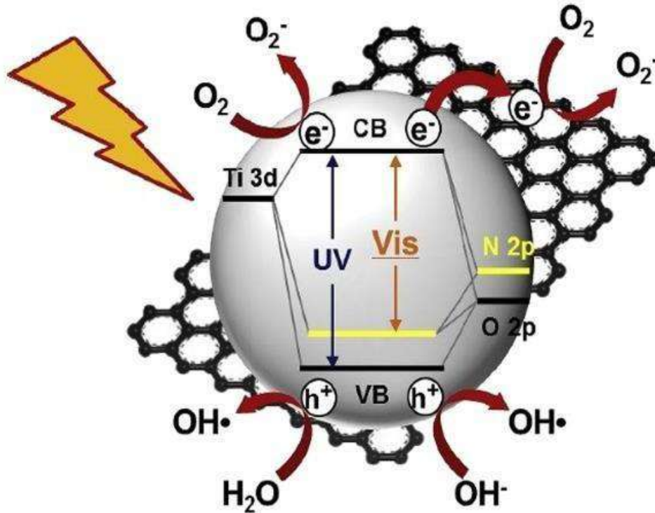
Figure 4: Schematic diagram of photodegradation mechanism
