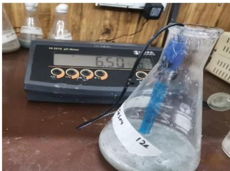
Figure 2.6: Adjustment of pH of fermentation media by pH meter at 6.5
